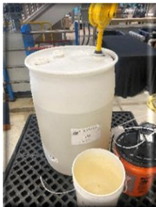
Figure 20: Lanthanum Storage. COMMENT: Use of lanthanum not effective to control algae at higher Phosphate Levels.
